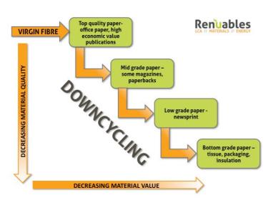
The very best quality paper is usually produced using chemical pulping of wood, yielding strong fibres that can be bleached to a very high level of brightness. This type of paper is used for office grade paper and for very high quality publications that have a long lifetime; it also forms a component of magazine grade paper. When paper is recycled, the fibres are damaged and it is more difficult to achieve such high levels of brightness and strength, so that
